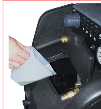
Add appropriate amount of chemical to water in solution tank
