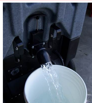
Drain water from Recovery Tank
